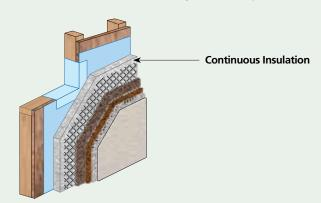
Continuous Insulation (C.I.) acts as the bond breaker replacing the separation sheet otherwise required over the water-resistive barrier. HE assemblies add a very light-weight energy efficient layer of insulation that allows building designs to meet new energy efficient building requirements such as Title 24 in California.
