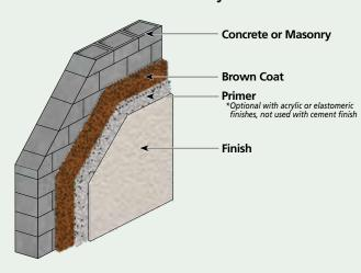
Designed for over either concrete or masonry walls where the aesthetic appeal of stucco is desired.
