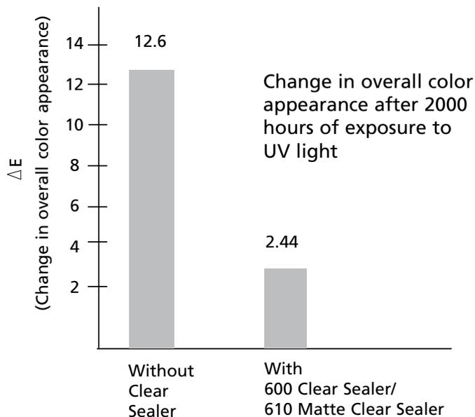
Finishes coated with 600 Clear Sealer/610 Matte Clear Sealer show far less change in overall color than finishes without 600 Clear Sealer/610 Matte Clear Sealer after 2000 hours of intense laboratory UV exposure. 600 Clear Sealer/610 Matte Clear Sealer keeps finishes looking fresher.
