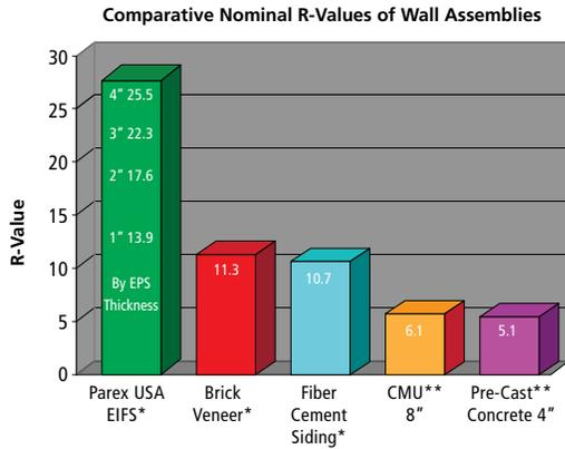
\* Includes 16" o.c. wood studs, R-13 stud cavity batts, 1/2" sheathing and wallboard.
