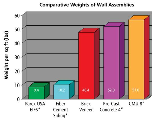
"Concrete Masonry Handbook for Architects, Engineers, Builders" PCA Portland Cement Assoc.
